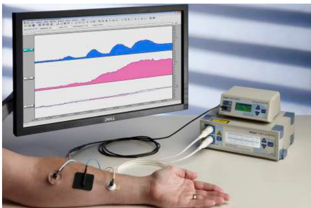
moorVMS-LDF2 and MIC2 – Experimental set-up with enhanced image of responses to simultaneous iontophoresis of Acetylcholine and Sodium Nitroprusside.
