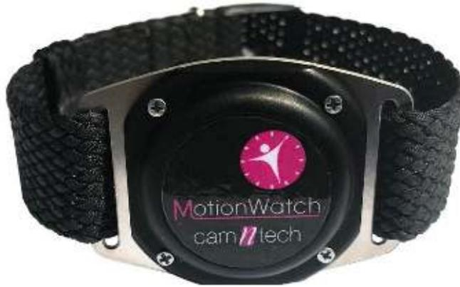
The MotionWatch R (Rugged) is a ruggedized version of the standard MotionWatch intended for use in harsh environments such as veterinary or military applications. The electronics are identical to the standard MotionWatch but the casing is all-metal to provide additional strength over the standard plastic casing. The Rugged case does **not** include the marker button or light sensor.
