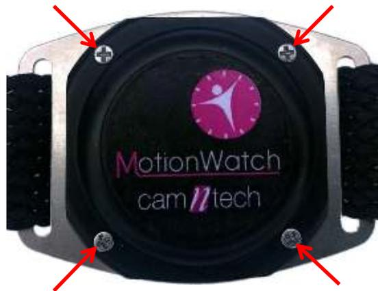
Gently lift away the front cover taking care not to lose or damage the O-ring seal. The electronics module is enclosed within a plastic housing (see photo below).
