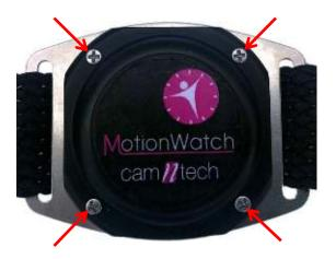
Gently lift away the front cover taking care not to lose or damage the O-ring seal.
