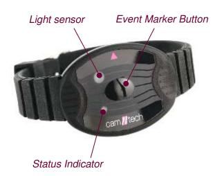
Event Marker: The MotionWatch has a front-panel button that may be pressed by the subject to mark specific events. Typically this will be used to mark when the subject goes to bed and when the subject gets up in the morning. The use of the marker will insert a date/time stamped mark within the data.
