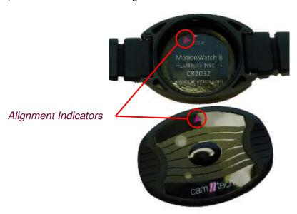
With the indicators aligned, drop the top part of the casing into the lower part and then turn clockwise by approximately 15 degrees to close.
