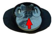
Note: Data will NOT be lost by removal of the battery.
