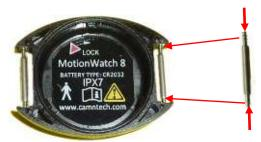
To remove the Strap: Use a flat bladed tool to gently depress one end of the spring bar by levering against the side of the casing. Take care not to damage the MotionWatch casing.
